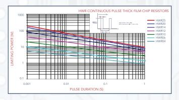
THICK FILM CHIP RESSITOR - HWR SERIES
