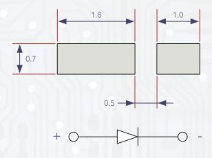
Reflow soldering should not be done more than two times When soldering, do not put stress on the LEDs during heating
